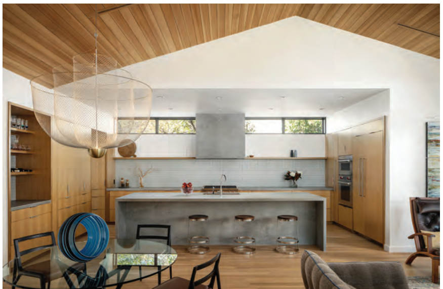
In the new family room, slot diffusers were seamlessly integrated into the hemlock ceiling with custom-routed frames that preserve the ceiling's uninterrupted appearance.
